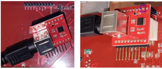
If you're connecting an older DL-20 display, then you will need to connect it to the output connector of the extender board like this:
