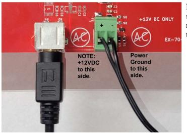
Now connect the other end of the supplied video cable to the EX-70-ASI main unit and connect the power like this:
